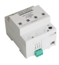
The MER12.5/24-48/DC provides economical and reliable class 1 protection for DC power distribution systems. nternal thermal disconnect devices ensure safe isolation during sustained and abnormal events on the distribution network, or at end of life. Visual indication and voltage free contacts are provided for remote signaling if replacement is due.
